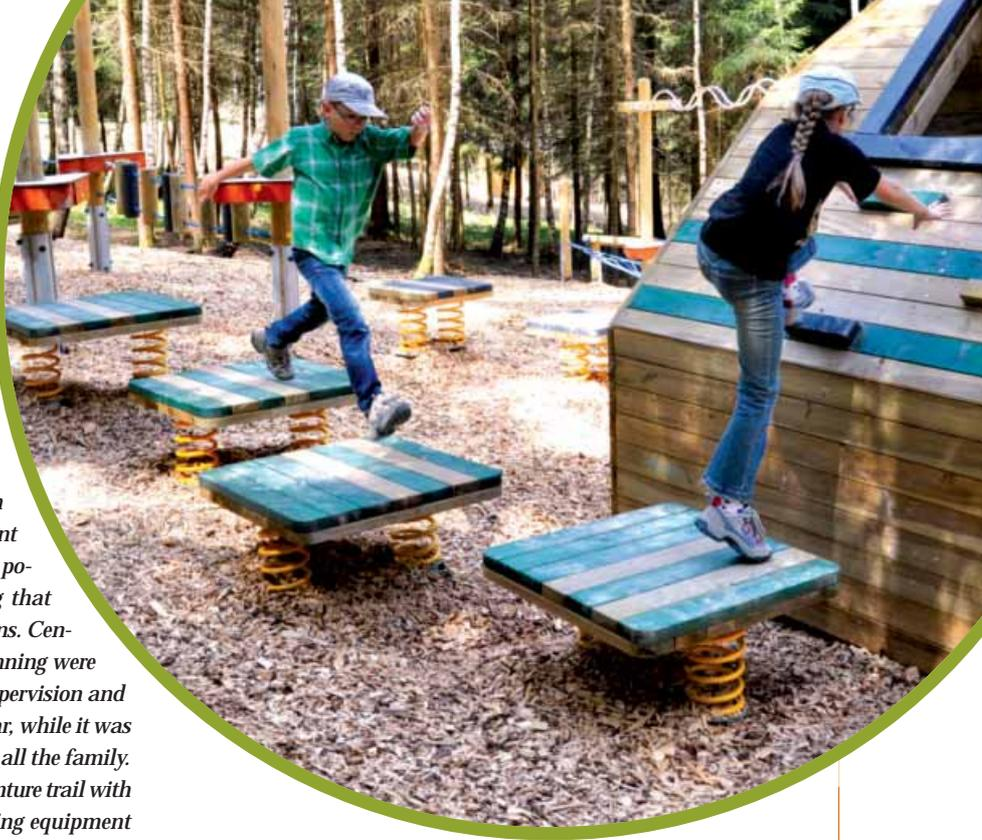
stainless steel for hanging and balancing systems and HPL with non-slip surface coatings for platforms. All posts are supported by steel plates and all wooden sections have been pressure impregnated to ensure maximum longevity.
